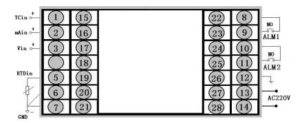
Note: The wiring diagram for the special model instruments, please refer to wiring diagram put on the instrument.
